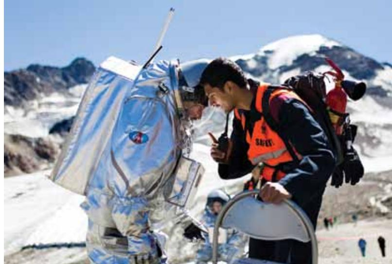
tional impact for astronauts would be. An Aouda suit weighs 45 kg, which is a good match for the weight of a future spacesuit on Mars (~135 kg, but approximately one third of this on Mars due to the lower gravity). It supplies ambient air and it supports biomedical and technical telemetry. An exoskeleton is used to simulate a pressurised suit on Mars.
