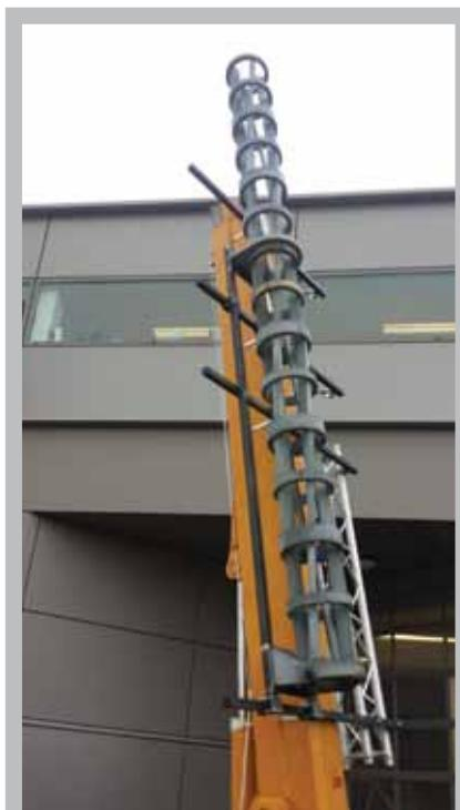
The Mobile launch platform with the guiding rail for the cansat launcher and the spiral tube for the DART.
