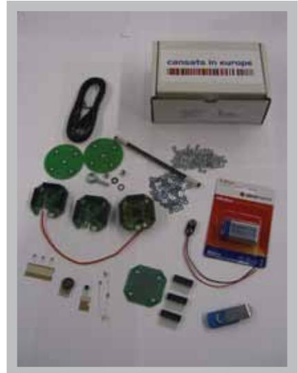
A CanSat kit including the basic components for a CanSat; a small board computer and transponder to send telemetry.
